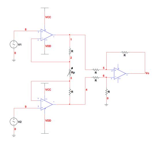
a) Obtain the expression for the circuit's input impedance, as seen by the voltage sources V1 and V2, considering the operational amplifiers as ideal devices.
